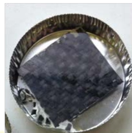
Composite sample before burn-off
