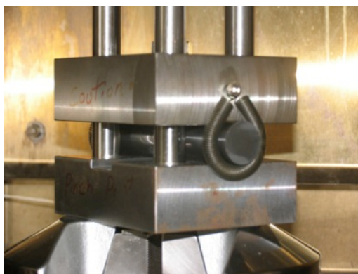
Die setup on the servo-hydraulic load frame
