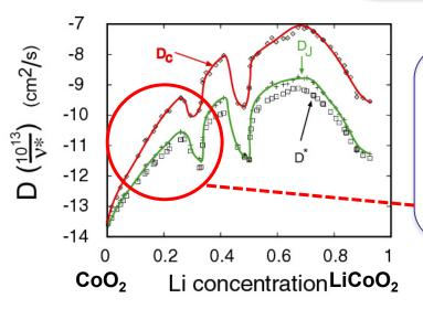
In layered materials slab spacing contracts at low Li concentration, thereby reducing Li mobility, and reducing practical charge capacity
