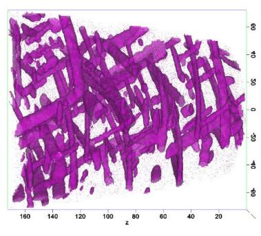
Local electron atom probe (LEAP) analysis of phase precipitation
