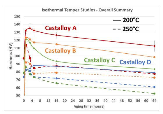
Hardness measurements on chemical buttons test temperature stability of four alloy concept models
