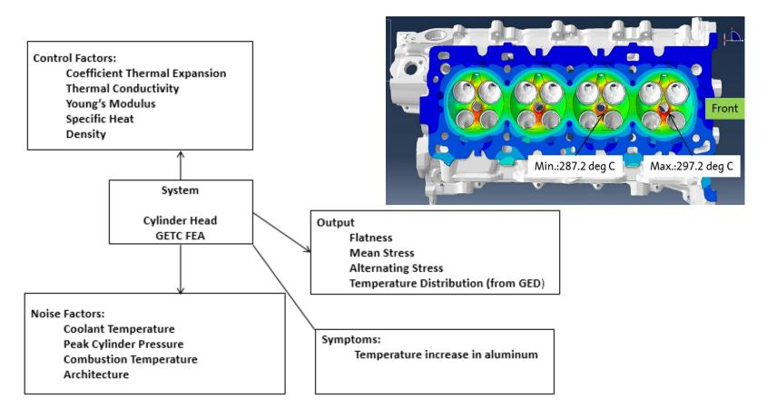
Apply Design for Six Sigma (DFSS) methodology to establish the most critical material properties to meet engine requirements
