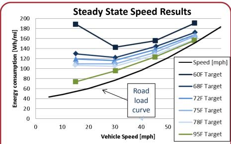
→ Use the AC at high speeds, but at low speeds the AC power outweighs the powertrain power
