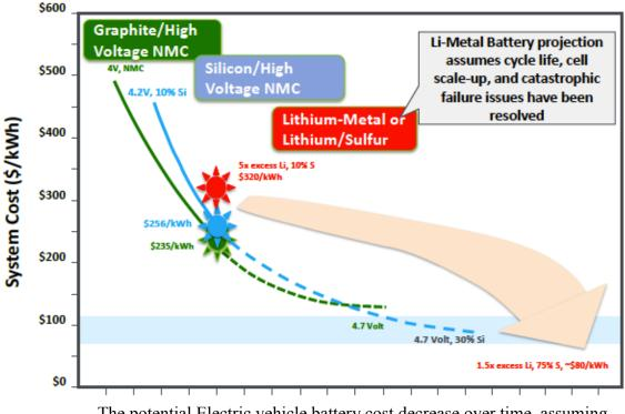
The potential Electric vehicle battery cost decrease over time, assuming successful research results in three technology areas
