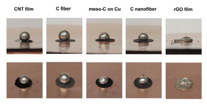
Figure 5. Example of various carbons' ability to incorporate Li metal. r-GO is being used as a Limetal host. Research from the Cui group at Stanford University.
