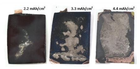
Figure 10. Images of graphite electrode in NMC622/Gr pouch cells. Lithium plating appears as metallic deposits on the surface of the electrode. Research from the Bloom group at ANL.
