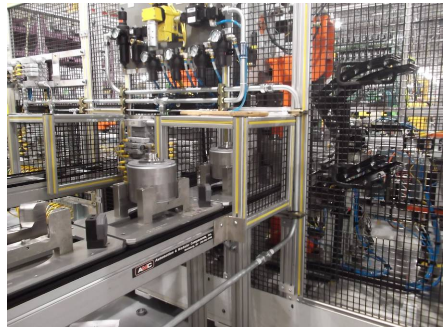
Rotors entering bearing press after magnetization
