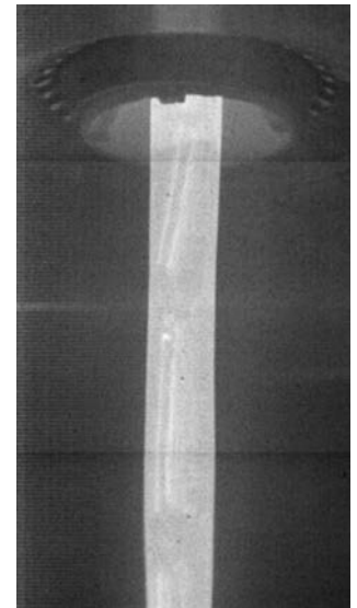
Melt stream before spray onset.
