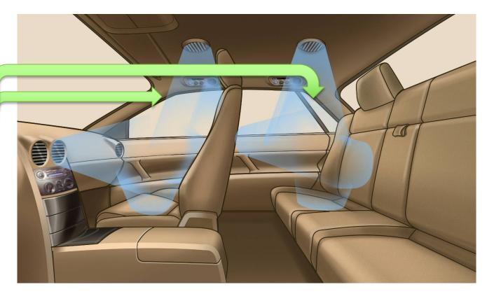
Zonal TE units located in dashboard, headliner, A&B pillars and seats/seatbacks
