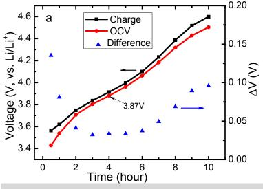
The Li half cell was charged/discharged at C/10 rate. OCV was taken after 3 hours rest.
