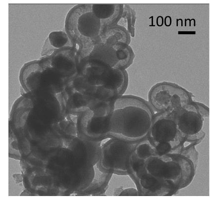
Si@hollow carbon nanocomposite
