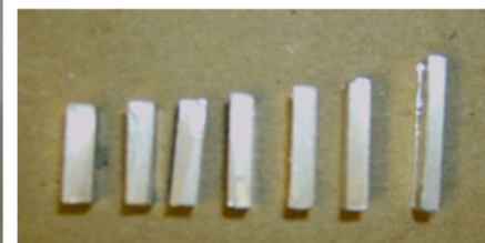
Extruded Specimens Deformed sheet samples (Stage VI)
