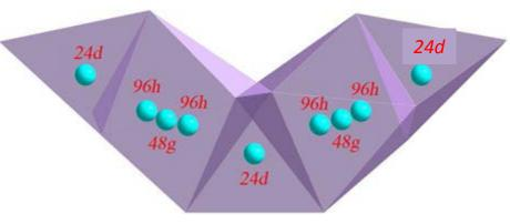
La<sub>3</sub>Ta<sub>2</sub>O<sub>12</sub> framework with Li in interstitial space
