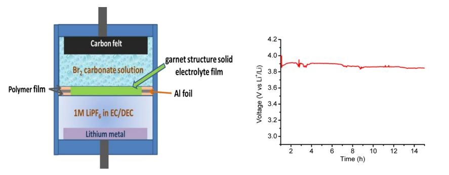
Garnet solid electrolyte is stable in bromine carbonate solution Bromine can be a very promising liquid catholyte for flow-through battery owing to its high open circuit voltage (4V) and high capacity (335 mAh/g) that is much higher than insertion compounds.
