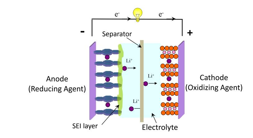
Capacity limited by Li solid solution in cathode and loss in SEI layer
