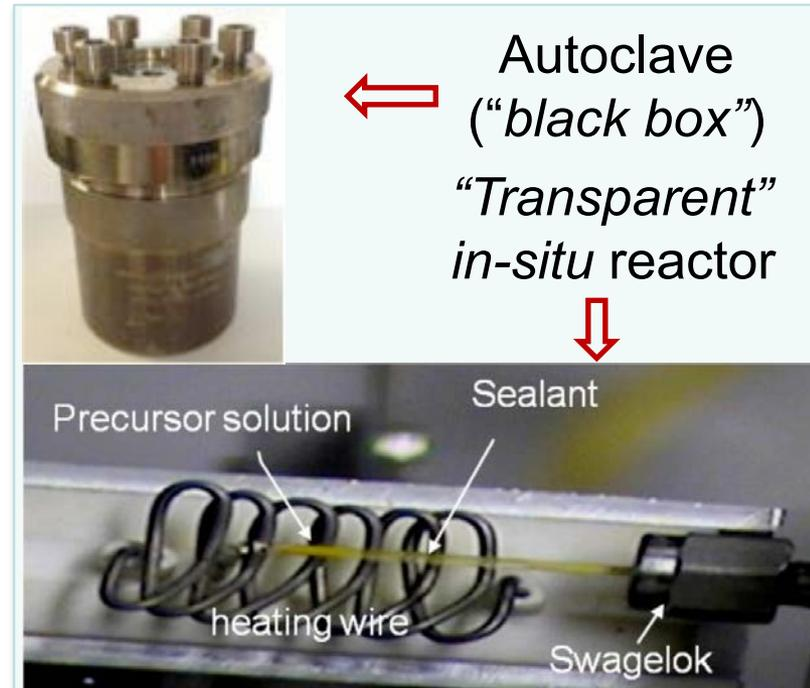
**Technique development** Explore reaction pathways and structural evolution of intermediates in real working conditions
