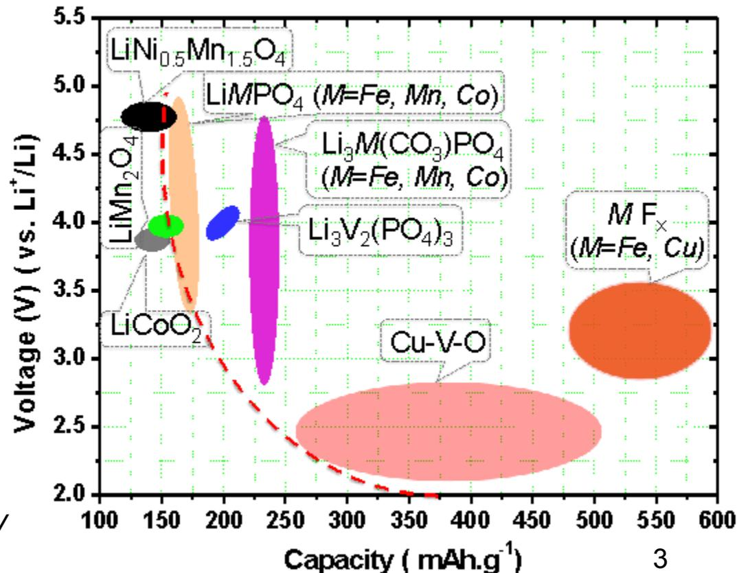
(\*Some cathodes with target energy density are given on the right side of the plot)
