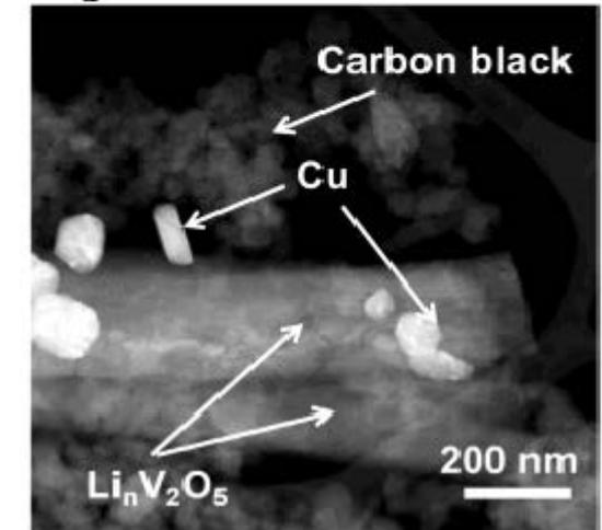
*Formation of large Cu particles on the surface of CVO rods with lithiation*
