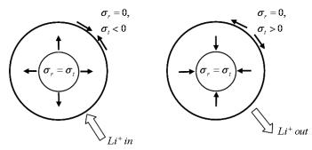
$$P_f(t) = 1 - \exp\left(-\int_V \left(\left(\frac{\sigma_r(r,t)}{\sigma_o}\right)^m + \left(\frac{\sigma_\theta(r,t)}{\sigma_o}\right)^m\right) dV\right)$$
