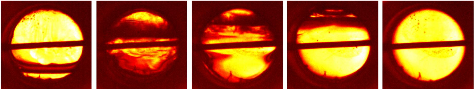
Diesel fuel-EGR flowing in a view cell from sub- to super-critical conditions of 394 °C and 229 bar
