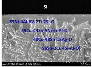
Die attach solder layer in Infineon HP1
