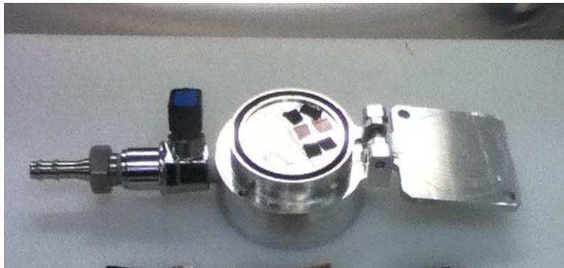
SEM vacuum sample holder for transfer of air-sensitive samples from glove box to SEM column
