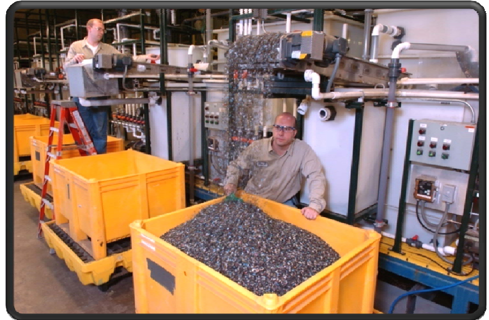
Argonne's Wet-Density/Froth Flotation Pilot-Plant
