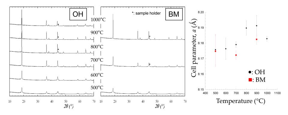
• Samples synthesized from hydroxide precursors: direct calcination for 12 h (OH, black), milling+calcination for 1-2 h (BM, red).
