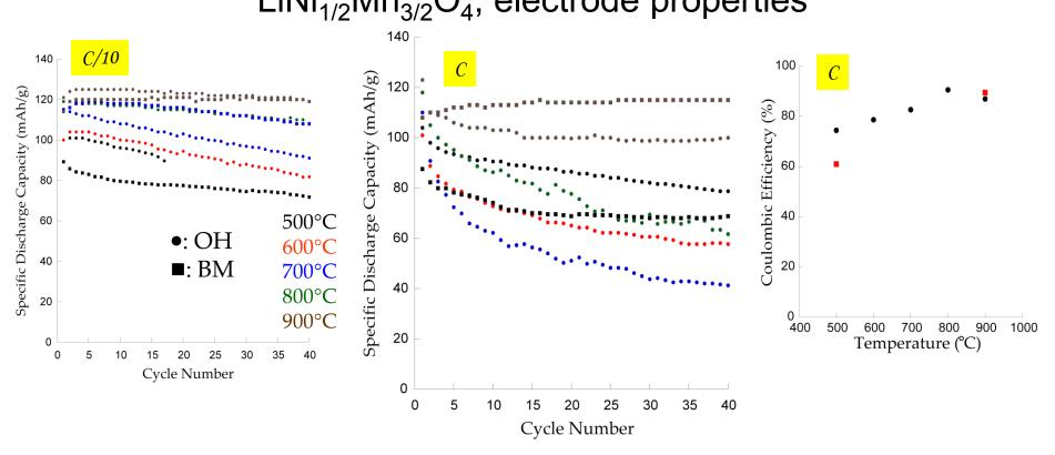
• Performance at moderate and high rates improves with synthesis temperature. <u>Particle</u> <u>size</u> seems to be **more critical** than <u>order-disorder</u> or capacity at 4 V (<u>Mn<sup>3+</sup> content</u>).
