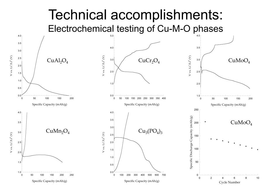
Cu extrusion at different V. Only reversible capacity for CuCr<sub>2</sub>O<sub>4</sub> and CuMoO<sub>4</sub>.
