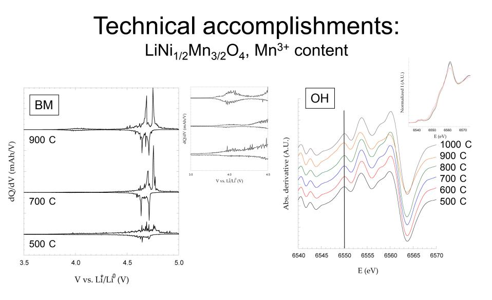
• Capacity at 4 V suggests presence of <u>different amounts of  $Mn^{3+}$ </u>, depending on synthesis temperature.
