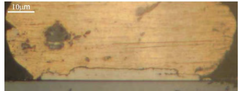
Intermetallic formation between Au wire and Al bond pad.
