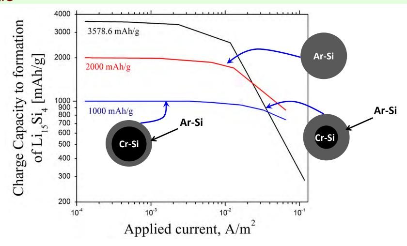
Capacity obtained determined by extend of cycling and by charge rate
