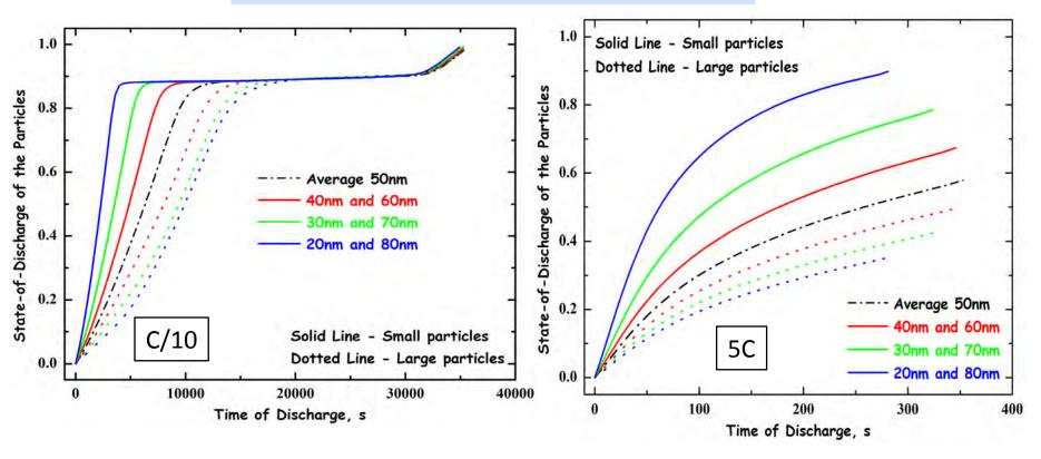
Small particles lithiate until singlephase region; large particles then "catch up" Transport losses result in deviation from the flat potential; less disparity in lithium content
