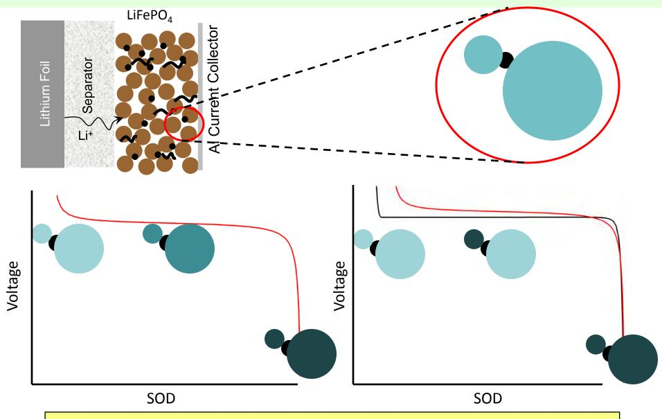
Disparity can exist in lithiation amount between particles of different sizes
