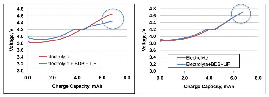
• Full cells NMC – hard carbon charged at 1C to 4.2 V then 0.1C to 4.7 V or 150% state of charge, whichever occurred first
