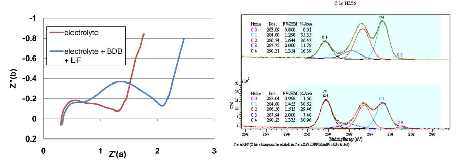
• Electrochemical impedance spectroscopy (left) and X-ray photoelectron spectroscopy (right) both show that the SEI layer is changed when formation occurs in the presence of the BDB redox shuttle molecule
