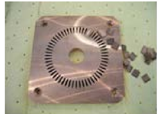
Rotor fabricated by Friction Stir Welding
