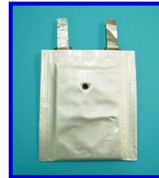
GCM/MCMB cell After test (thermal runaway)
