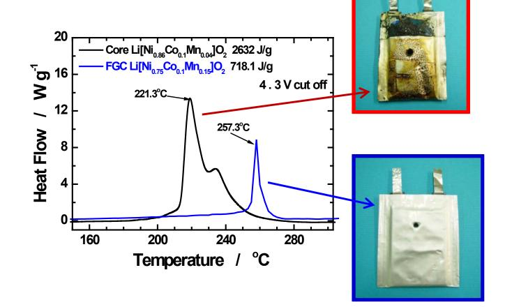
FGC material shows high onset temperature and 3 times lower heat flow than the core composition
