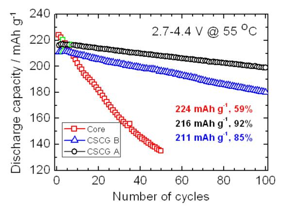
Gradient cathode that has the highest Mn content on the outer shell of the particle (CSCG A) shows better cycling performance than the one with less Mn content on the outer shell of the particles (thought the later has thicker shell thickness).
