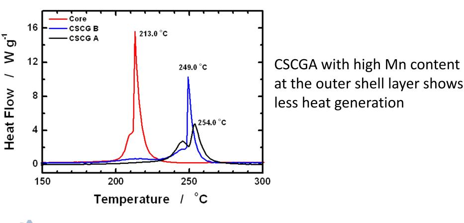
High Energy Full Gradient Concentration Materials (FGC) with average composition LiNi<sub>0.6</sub>Co<sub>0.10</sub>Mn<sub>0.30</sub>O<sub>2</sub>
