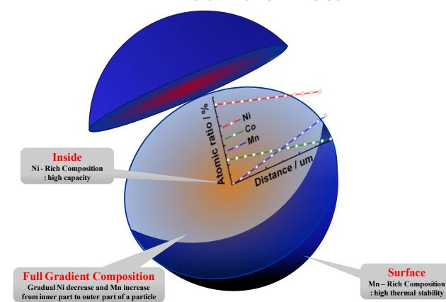
Schematic diagram of the full concentration gradient lithium transition metal oxide particle with the nickel concentration decreasing from the center toward outer layer and the concentration of manganese increasing accordingly.
