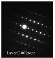
Electron diffraction of pristine core showing layered phase
