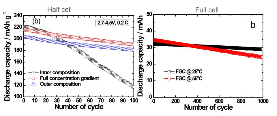
Full concentration gradient shows high capacity and very limited capacity fade after 1000 cycles at 55°C in a full cell, Electrolyte used is  $LiPF_6/EC:EMC$  with 1%VC
