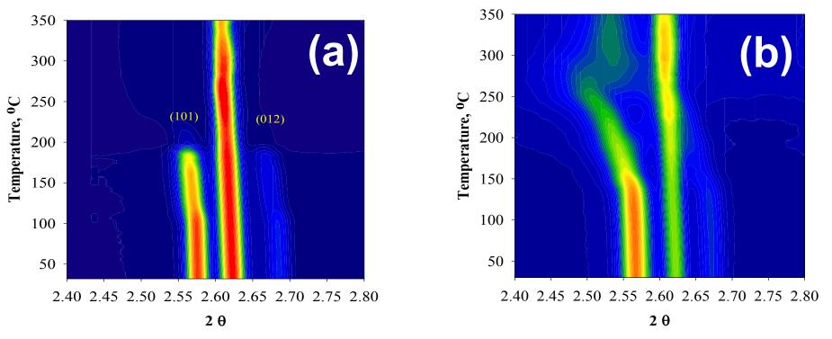
Contour plots of in situ high energy X-ray diffraction profile of (a) delithiated core composition material [Li<sub>1-x</sub>(Ni<sub>0.86</sub>Co<sub>0.10</sub>Mn<sub>0.04</sub>)O<sub>2</sub>] and (b) delithiated FGC material during thermal ramping from room temperature to 375°C with a scanning rate of 10°C min<sup>-1</sup>
