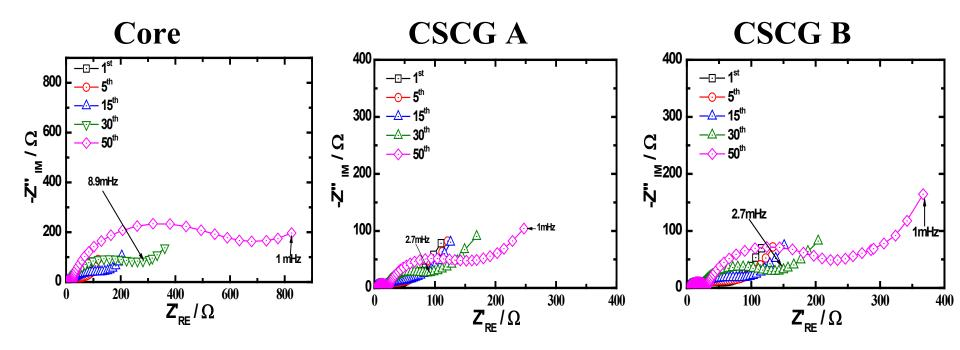
(CSCG A) with shorter shell thickness but high Mn content at the outer shell layer of the particle shows less impedance growth during cycling at 55°C.
