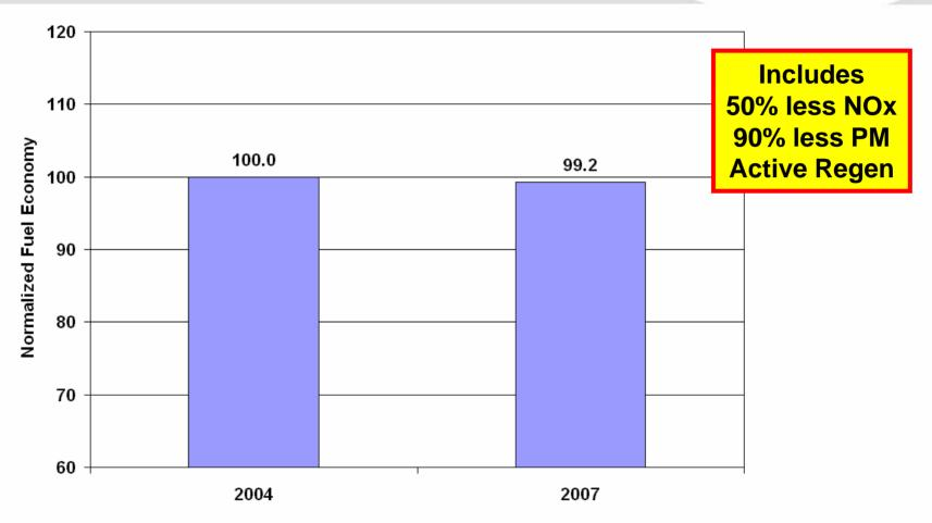
Testing showed EPA07 engine to be within 1% of the EPA04 engine. All runs were within 2% variance.
