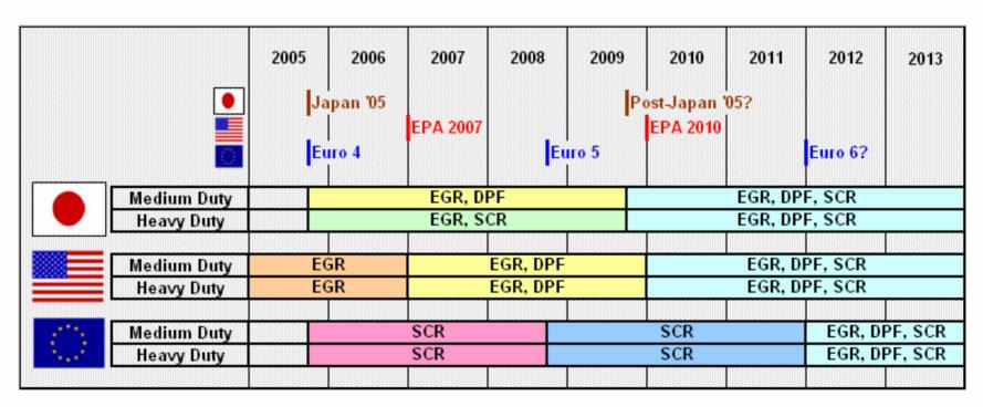
Production experience with several emissions control technologies within the DC family (e.g. EGR in U.S., SCR in Europe) lays a strong foundation for a global solution
