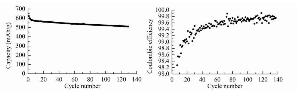
Milestone (b) achieved using method 1: Tin-carbon electrode + Fe as Sn<sub>2</sub>Fe
