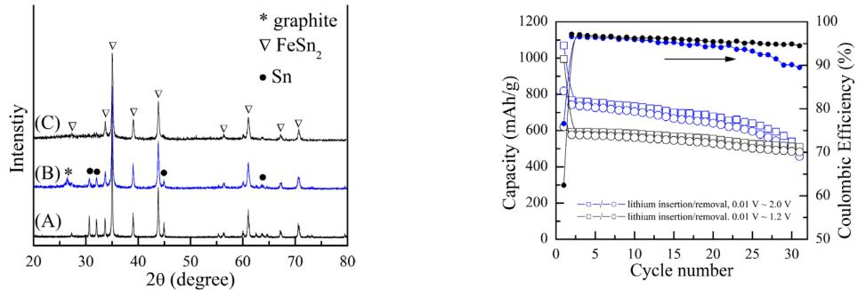
(left) XRD patterns of (A) Solvothermally formed Fe-Sn; (B) Planetary ball-milled (pBM) Sn-Fe-C composite; (C) High-energy ball-milled (HEBM) Sn-Fe-C composite. Sn metal phase in the solvothermally formed material disappears after high-energy milling with graphite. (right) Electrochemical cycling of this Sn-Fe alloy in two voltage windows; no grinding with carbon. The current was 0.3 mA/cm<sup>2</sup> in the 1<sup>st</sup> cycle and then changed to 0.5 mA/cm<sup>2</sup> thereafter.
