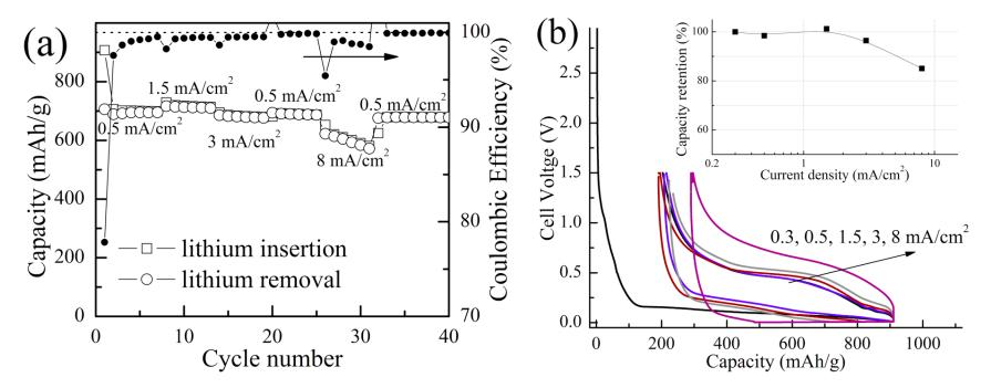
Rate capability of SMOG electrode between 0.01 V and 1.5 V. (a) capacity on cycling at different current densities; (b) cycling curves at different rates, and Ragone plot for Li insertion. 1 C rate = 2.8 mA/cm<sup>2</sup>. The first cycle current density was 0.3 mA/cm<sup>2</sup>.
