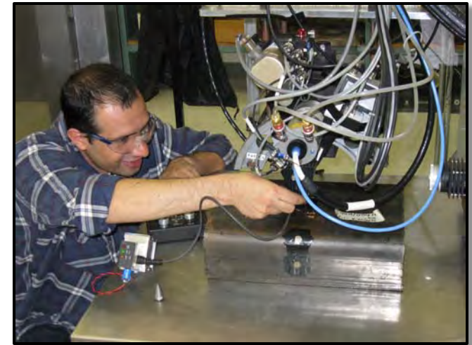
Metalsa’s Joaquin del Prado Villasana prepares for an X-ray diffraction measurement
