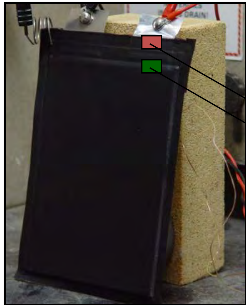
15 A-hr enclosed in pouch used for this study
