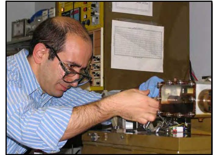
Dr. Omer Cora (VCU) preparing a test using a reciprocating cylinder-on-flat configuration .
