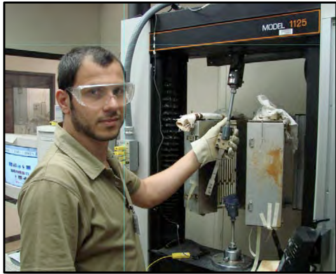
VCU's İrfan Kaya mounting a sample for high temperature tensile testing
