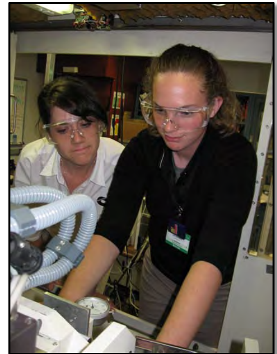
Madeleine Smith and Lisa Behrens of Cummins mounting a test specimen for X-ray diffraction measurements
