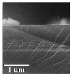
Near-frictionless Carbon: -Friction coefficients down to 0.001 feasible -Excellent compatibility with alternative fuel environments
