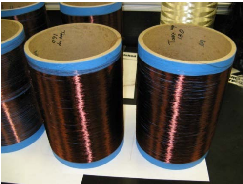
Processed Precursor Fibers from a Hardwood/Softwood Lignin Blend.
