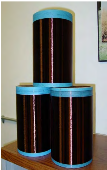
12-filament fiber spun from Kraft hardwood lignin
