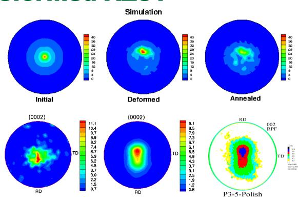
Spreading of the basal texture to off-basal orientations
