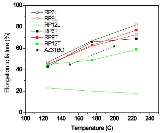
RP6 and RP9 show slightly better ductility compared to 1 mm thick AZ31B-O sheet tested in prior work
