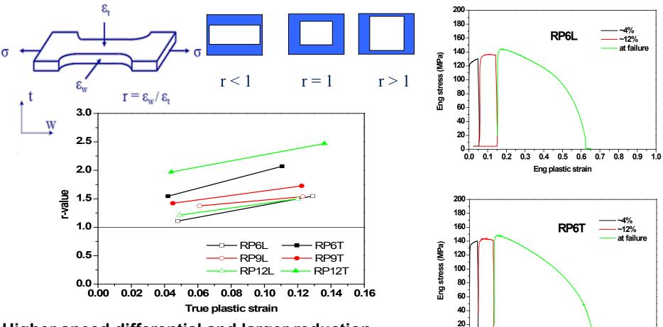
Higher speed differential and larger reduction (RP12) results in higher anisotropy in r-values
