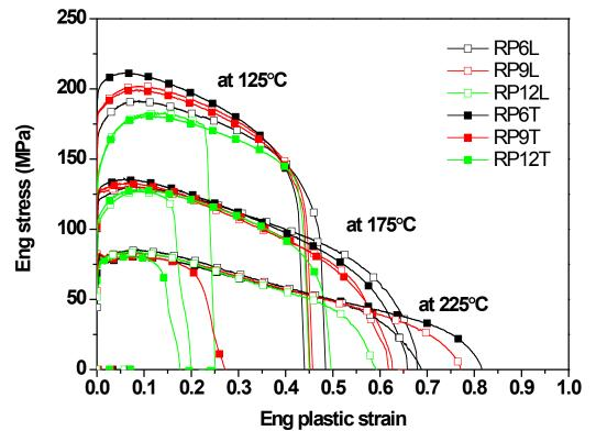
Yield Strength of RP12 is lowest at 125°C and 175°C but has lower ductility in the as-rolled condition
