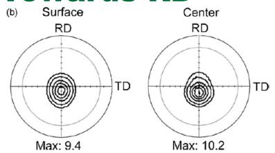
Fig. 3. (0002) pole figures of (a) the normal rolled sheet and (b) the DSR processed sheet measured at the surface (left part) and the center (right part). Intensity levels: 1, 2, 4, 6, 8...
