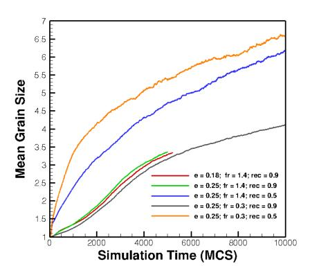
Rec= Recovery/Recrystallization e= Plastic True Strain f= Shear Stain/Compression Strain
