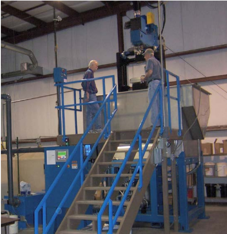
Figure 2. (A) Overview of the 20-foot tall, pilot-scale 3-DEPT TM machine. (B) Detail of the forming head of the 3-DEPT TM machine showing the forming screen for an automotive "B-pillar" (used in the Phase I project) and the four degrees-of-freedom (roll, pitch, yaw, and z-translation) that provide the unique forming capability of the 3-DEPT TM technology.
