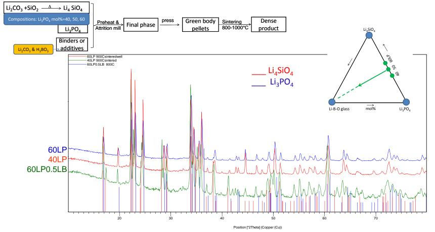
•  $xLi_3PO_4$ ·(1-x) $Li_4SiO_4$  (x=0.4-0.6) synthesized by classical solid state method. Addition of LiBO<sub>3</sub> as sintering agent.
