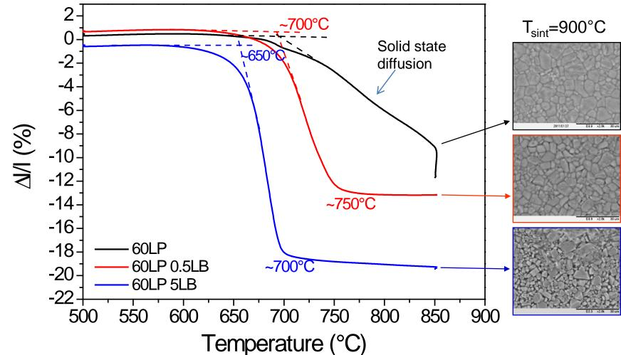
• Addition of LiBO<sub>3</sub> enhances sintering and lowers densification temperature.
