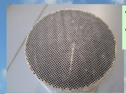
5"66 diameter, 6" length, 180cpsi, 19 μm mean pore diameter, 50% porosity
