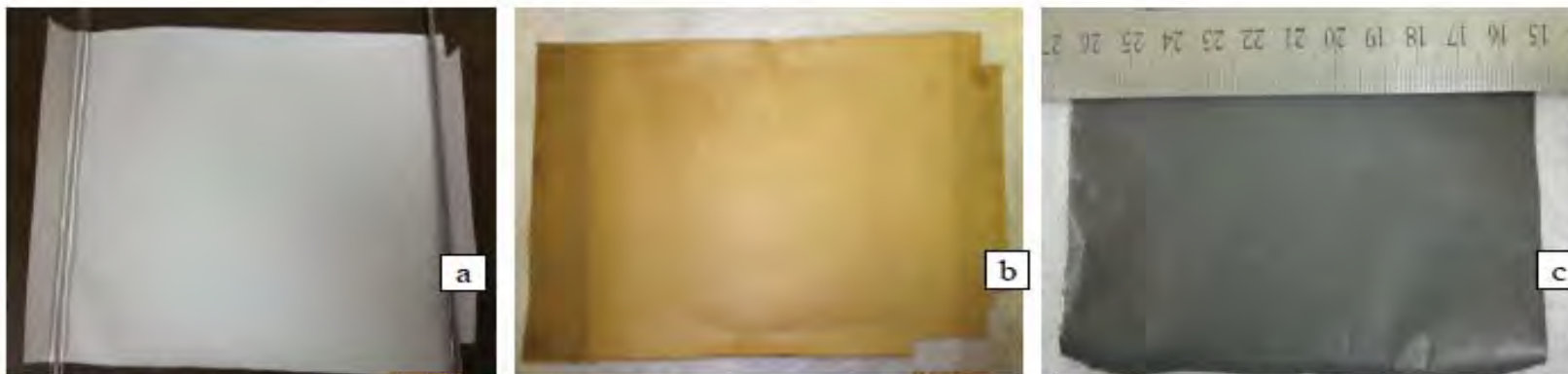
Figure 2. Optical images of a laminated structure anode electrode during different stages of the heat treatment process: (a) as-made, (b) pre-oxidized, (c) after carbonization.
