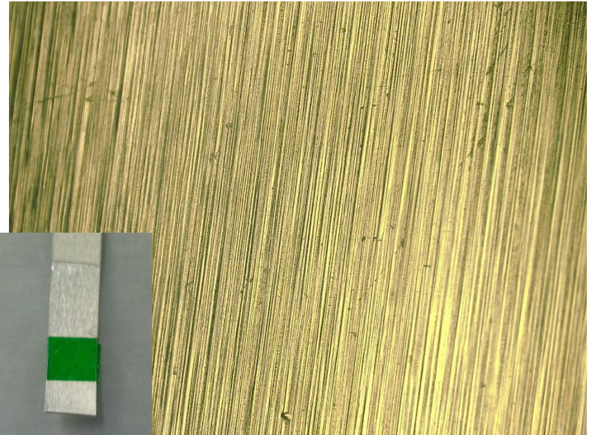
Pristine Al electrode using HV salt
