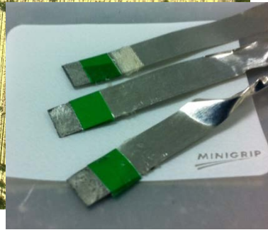
Corroded Al electrode using Baseline salt
