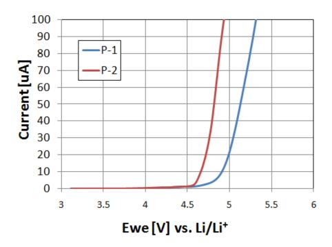
Cyclic Voltammetry of catholyte polymers P-1 and P-2. Carbon working and counter electrodes used with Li metal reference
