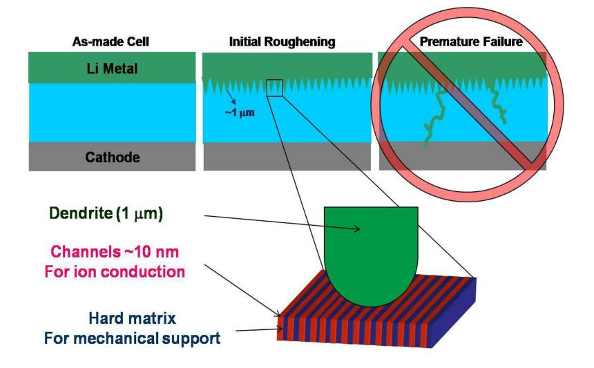
Schematic of the mechanism of dendrite growth inhibition by Seeo's solid polymer electrolyte
