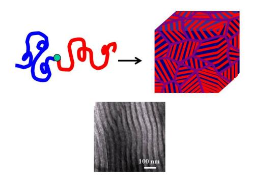
Self-assembly of block copolymer electrolytes and TEM of nanostructured electrolytes.
