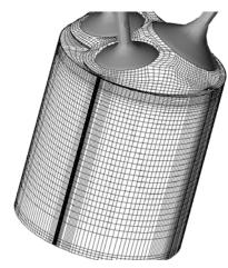
1. KIVA3V with CHEMKIN calculations in every cell: *months* in 100 processor computer. For benchmarking only
