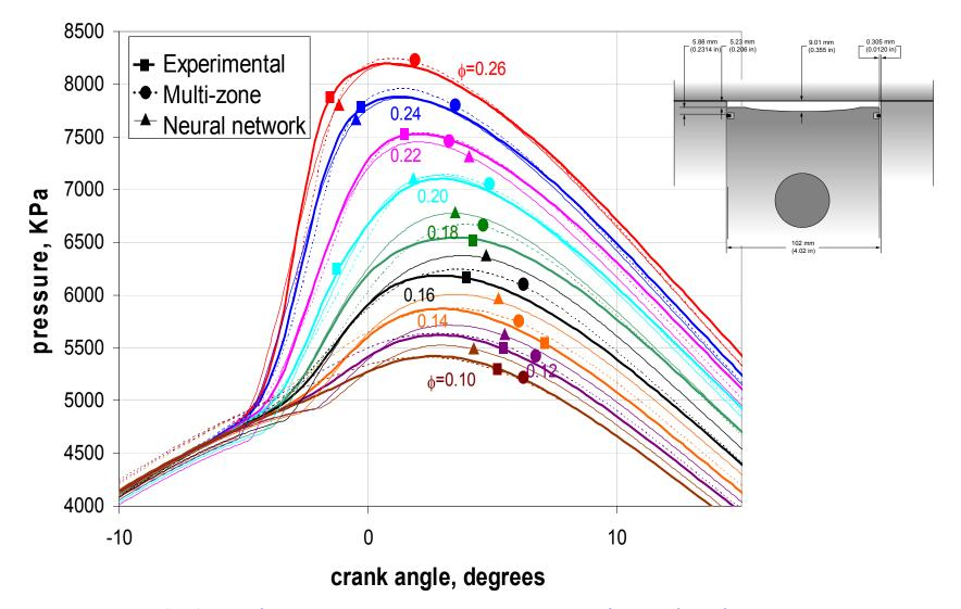
KIVA-ANN is almost as accurate as detailed kinetic models while considerably reducing computational cost (4 hours for 50,000 element mesh) Our ANN has been trained over a broad range of  $\phi$ -EGR enabling fast and accurate analysis of partially stratified combustion
