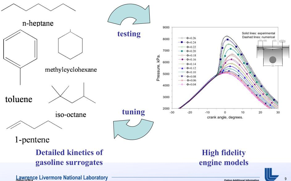
We develop & refine surrogate gasoline chemical kinetic models by producing detailed mechanisms for all the major chemical classes
