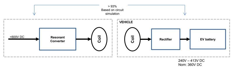
Circuit Simulation Model of power transfer efficiencies from DC Charger input to DC Receiver output to EV battery
