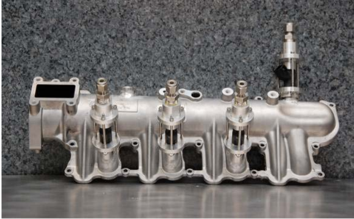
Modified intake showing PFI injectors. Cylinder 1 is offset due to high pressure pump interference.
