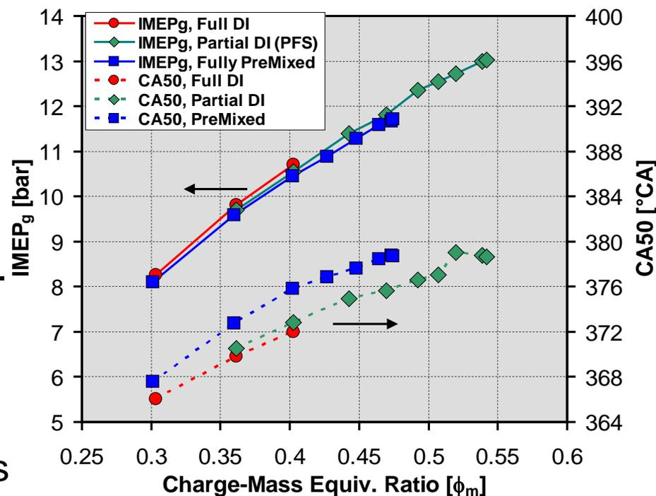
• PFS allows a large increase in load for gasoline boosted to  $P_{in} = 2$  bar.
