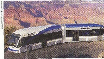
North American Bus Industries' (NABI) 60-BRT is a common articulated bus for public transport in major cities. A number of the auxiliary systems, including the air conditioning, are located on the roof of the bus under access doors similar to that used in the UAB/NCC project.
