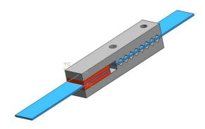
**Figure 4.** High strain rate lap-shear specimen for L&L Products.
