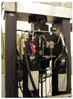
**Figure 8.** Accumulators and servovalve for high strain rate test machine.
