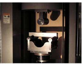
Figure 2. Three-point-bend test setup on TMAC.
