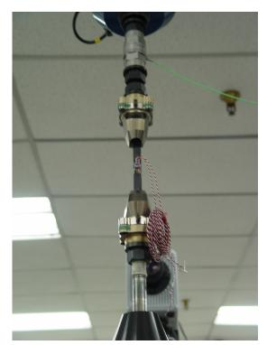
**Figure 5.** Typical coupon test setup on high strain rate tension machine.
