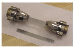
**Figure 9.** Low-mass grip used in high strain rate test machine.
