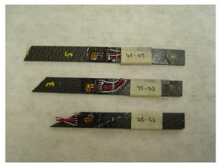
Figure 6. Typical failed off-axis tension specimens.
