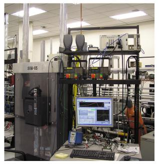
**Figure 7.** High strain rate (18 m/s) coupon test machine.
