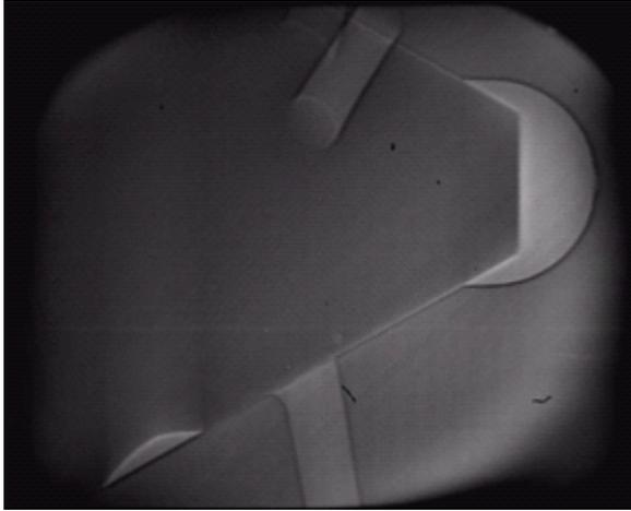
High-speed x-ray imaging of pintle motion was developed in 2004
