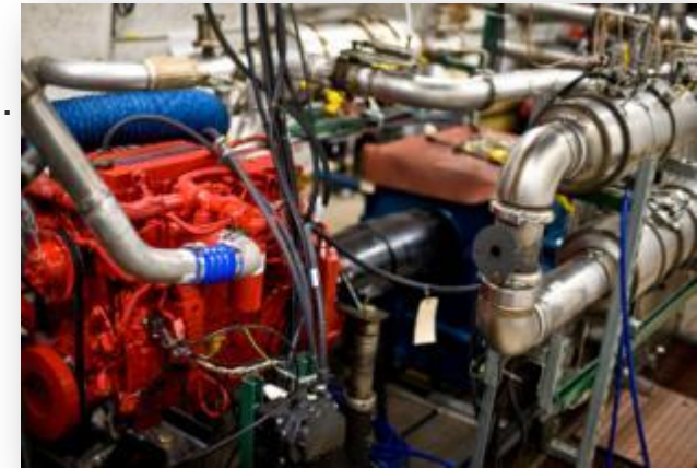
Cummins 2010 6.7L I6 ISB engine with ECU control and full aftertreatment system
