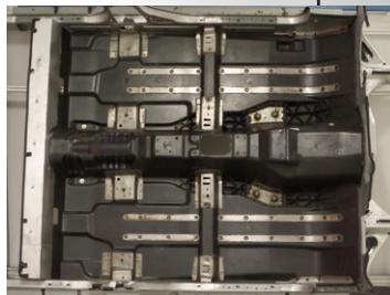
The Automotive Composites Consortium Structural Composite Underbody project led to the rapid commercialization of the Chevrolet Spark EV battery enclosure. (Courtesy of General Motors and the National Renewable Energy Laboratory.)
