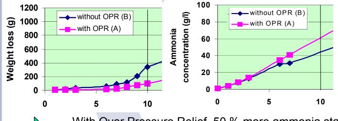
With Over Pressure Relief, 50 % more ammonia stays in solution and can be injected in the exhaust line
