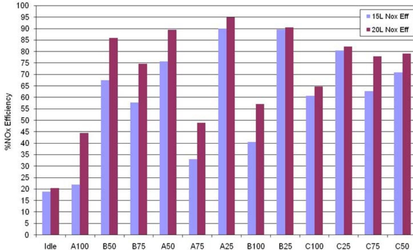
**Space velocity, oxygen concentration and gas temperature each contribute to the NOx conversion at a give engine operating point**
